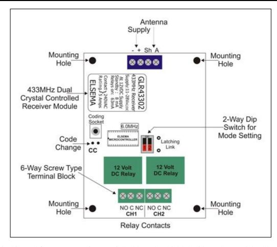
Sh terminal is used for antenna's using coaxial cables. The shield (braid) on the coaxial cable should be connected to the Sh terminal while the core of the coaxial cable is connected to the A terminal.
