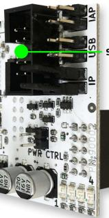
**Serial Port** - For use with USB-D-LINK upload/download cable for firmware upgrades, saving panel config, PC programming & review
