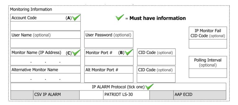
After completing the network set up (as explained on the previous page), you are required to enter the 'CID Settings' section. This is where you are required to enter the information gathered from the monitoring station. See below:
