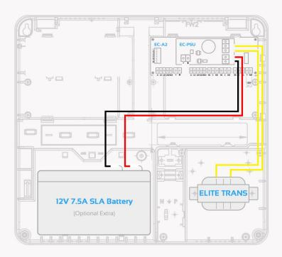
**EC-SCC BATT** - Optional battery holder for structured cabling cabinets. Ideal for mounting SLA batteries directly above or below the power supply
