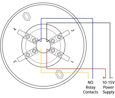
The relay contacts can be changed to be Normally Closed (NC) by opening the cover and moving the jumper to the NC pins. Please note this is not recommended as if the smoke is put on the base incorrectly the contacts could short out the power supply.
