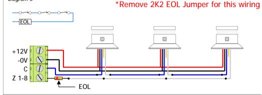
Multiple Detectors in Series Connection (using N/C Contacts) Individual wiring
