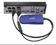
Signal Strength: A Fast flashing Blue Light on the Slave Adapter indicates good signal strength.
