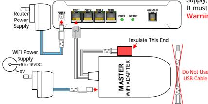
If the Router has neither a USB port or compatible Power Supply, a separate Power Supply is required.
