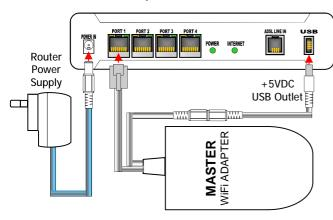
If the Router has a USB port you can use this to power the Master WiFi Adapter, Simply plug it in.
