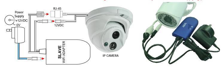
Master Connection Option 4: Adding an IP Camera Plugging the Master Wifi Adapter into a NVR Camera Port will allow the Slave Wifi Adapter (as shown above) to be found by the NVR. For Master connect as shown below
