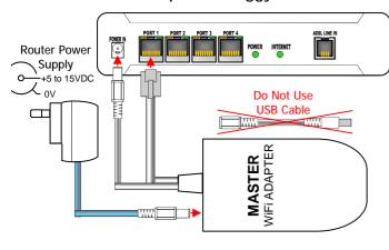
If the Router is powered using a 5 to 15VDC power supply with 2.1mm DC plug (positive centre)
