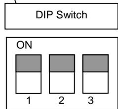
In the drawing above the DIP switches are indicating that the RS232 board is set to keypad address number 8 (switches 1, 2 & 3 all ON). Switches 4-8 are unused.
