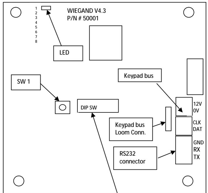
When the RS232 board is connected to an ELITE-S control panel the LED on the board will flash at approximately 1/2 second intervals to show it is working.
