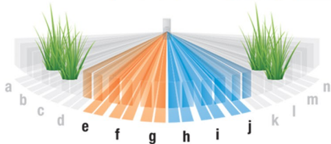
When area masking shutter's position is that Left is d and right is k, detection area a-d and k-n are masked.
