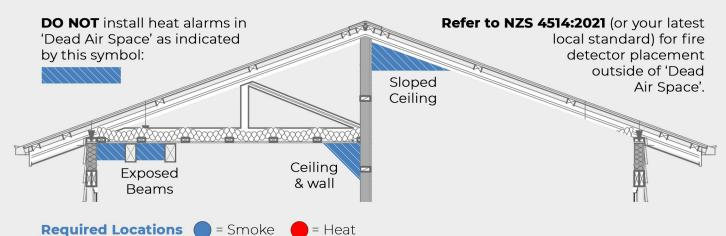
Interconnected heat detectors are to be installed in areas such as kitchens which can be closed off from the rest of the house (as detailed in the diagram below). This will help to avoid nuisance alarms in cooking and other similar areas of a house.
