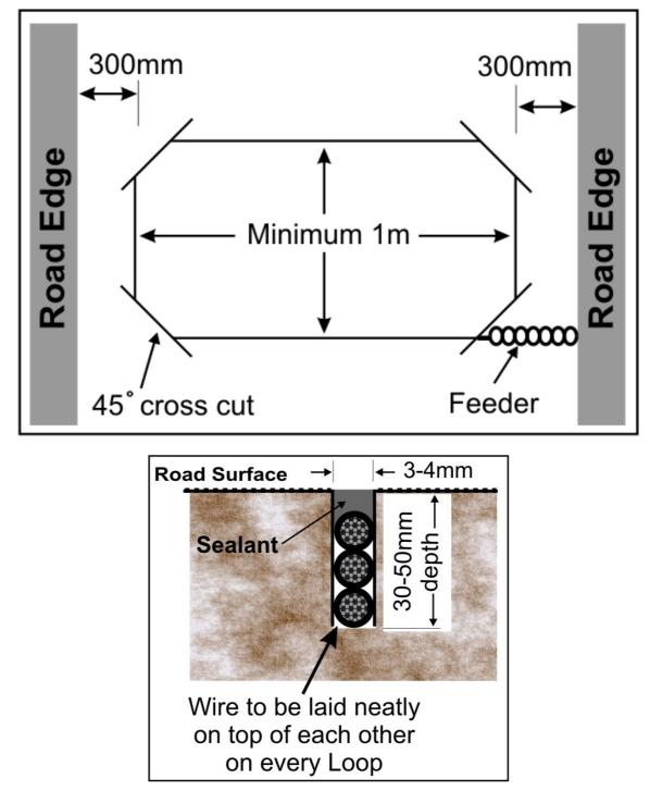
Once complete, seal the loop slots with epoxy compound or bitumen filler. (It is recommended this is only done after the detector has been connected and tested).
